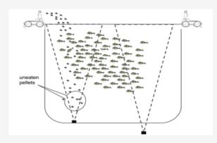
Acoustic technologies and devices for biomass and feeding control in floating cages for intensive aquaculture. Through an echo sounder system, continuous non-invasive monitoring of growth, quantification of uneaten feed, estimation of biomass density, and escape alerts can be performed.
