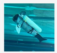
Detachable sensor carrier designed for measuring greenhouse gases in aquaculture facilities. It can be mounted on the fish-robot but also used independently via a LARS (Launch and Recovery System), providing added versatility.
