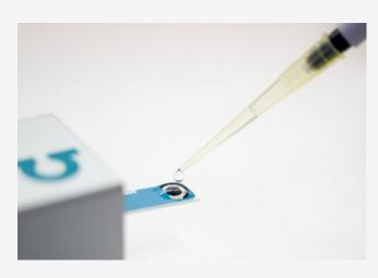
Electrochemical environmental alert device for rapid detection of chemical-biological risks in farming areas. The low-cost, portable, and easily integrable device allows for sensitive and rapid measurements, facilitating early warning generation without the need for specialized technical personnel.
