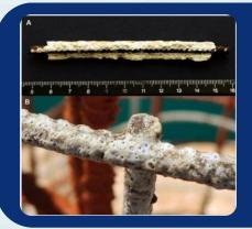
A hard calcareous coating (calcite and aragonite) has been created on steel mesh, strongly adherent and rough (favoring larval attachment) of variable thickness depending on the intensity of the direct current (general, photovoltaic). This has given rise to the utility model: PT/es2021/070734.
