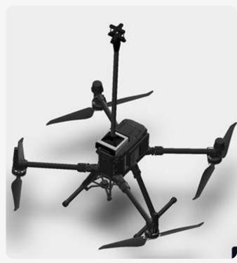
ThinkInAzul has developed a cost-effective "Meteo-Dron" to establish a high-resolution spatio-temporal monitoring system for atmospheric variables (wind direction and speed, air temperature, humidity, and atmospheric pressure) within the mid and lower troposphere (up to 5-7 km). The "Meteo-Dron" is built around a Matrice 350 RTK device equipped with a LI-550 TriSonica sensor.
